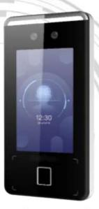
WTD-UF341FP face recognition terminal adopts deep learning algorithm, which helps to recognize the face faster with higher accuracy. It also supports multiple authentication modes: face/card/fingerprint authentication, etc. It can be applied in multiple scenarios, such as buildings, enterprises, financial industries, and other important areas.
